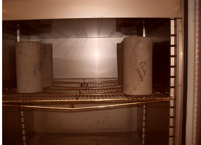
Figure 7.1: Concrete Specimens placed in Oven
