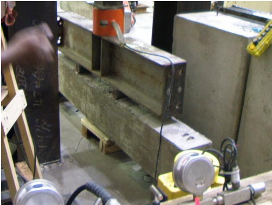
Figure 8.32: Experimental Results for the TDA concrete (7.5%TDA) Beam. The Beam with TDA did not fall into two halves.
