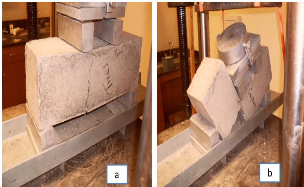
Figure 4.7: (a) Failure pattern for 7.5% TDA -1" concrete beam. The beam did not fail into 2 halves and fracture line was not parallel to loading direction (b) Failure pattern for Control-0% TDA concrete beam. The beam failed into 2 halves and fracture line was parallel to loading direction.
