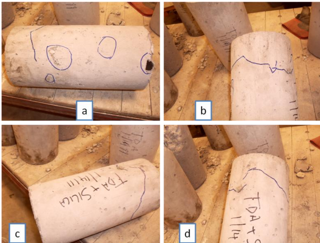
Figure 7.5: Cracks and spalling on TDA Concrete with Silica Fume after exposure to 100°C for 3 hrs in the oven.
